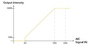
It is possible to control the light output between 10% and 100% of the max value with the AIC pin.
