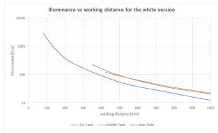
**Notes:** Measurements were made with a 2000mA strobe current through each LED (MX2). Please refer to the Power factor array for more information.
