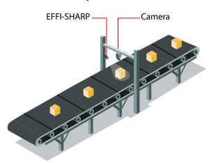
Tangential illumination for carved codes reading, cleavage inspection, edges view enhancing
