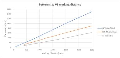
**Notes:** Measurements were made with the disc  $\emptyset$ 15,1 mm mask (Z=2).
