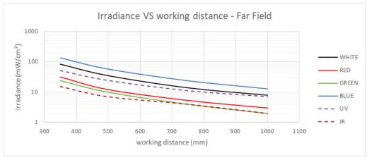
**Notes:** Measurements were made with a 2000mA strobe current through each LED (MX2). Please refer to the Power factor array for more information.
