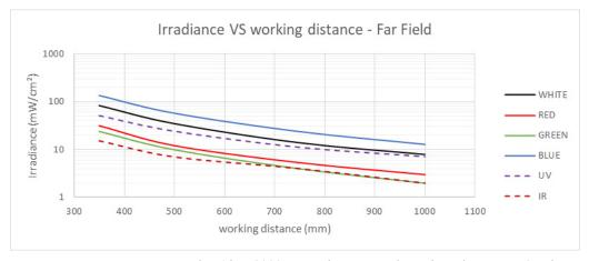
**Notes:** Measurements were made with a 2000mA strobe current through each LED (MX2). Please refer to the Power factor array for more information.
